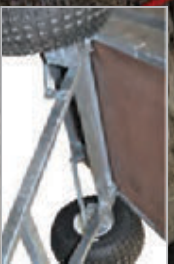
Spring assisted tipping mechanism.
