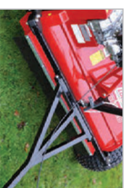
This model has a simplified drawbar and is towed in the central position.
