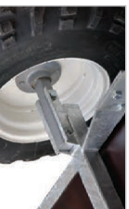
Bolt-in stub axle to allow easy maintenance or replacement when the time comes, without disturbing the galvanising protection.
