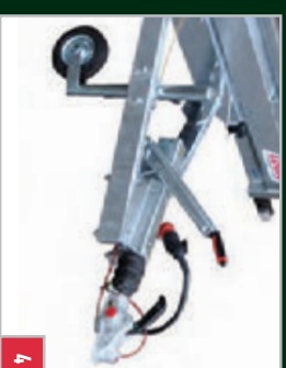
Overrun brakes with safety breakaway cable, handbrake and jockey wheel.
