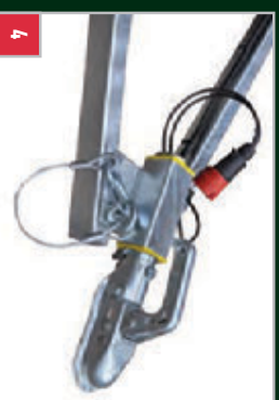
Attachment to the towing vehicle features a high quality coupling, heavy duty restraining cable, 7 or 13 pin electrical plug with storage socket and drawbar skid.
