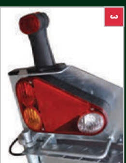
Protected light cluster with inbuilt triangle, lenses and marker lights.
