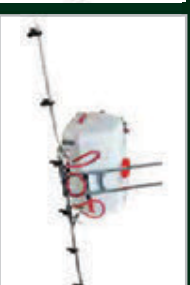
OBS135S 135 litre flat bottomed base sprayer with OBS104D 3.0 metre boom. Ideal for UTVs or compact tractors.
