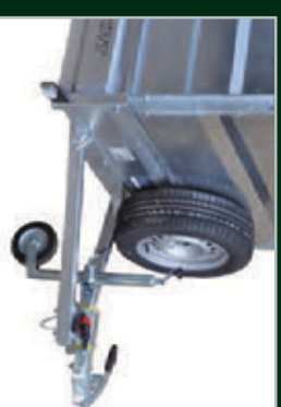
Other options include a spare wheel with WB103 mounting bracket and RT7710-01 jockey wheel.
