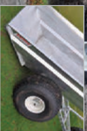
Optional WT510 turf tyres (right) offer non-marking tyres for use on delicate grass surfaces.
