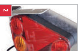
Protected light cluster with inbuilt triangle and lenses.
