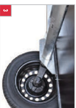
Standard AL-Ko axle with progressive rubber suspension giving an excellent smooth, quiet ride.
